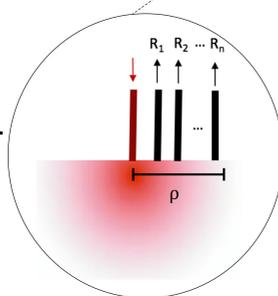
Figure 2. Conceptual scheme of a reflectance probe.
