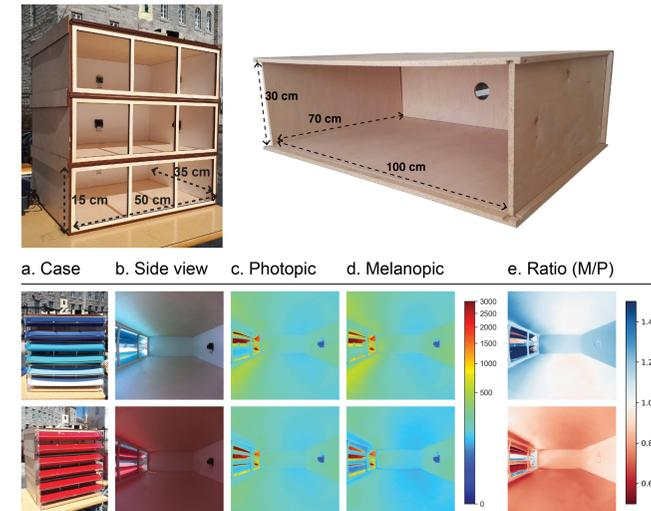
Figure 4. Scaled models and examples of computational lighting analysis
